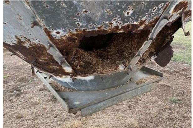
*Fiberglass silos do not corrode! Salt and ammonium in the feed, combined with water condensation, result in corrosion, which composite materials are resistant to.*
